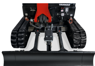
Extended undercarriage: 1170 mm
