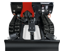
Retracted undercarriage : 980 mm
